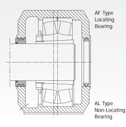
Housing for shaft end, (locating and non-locating bearing
